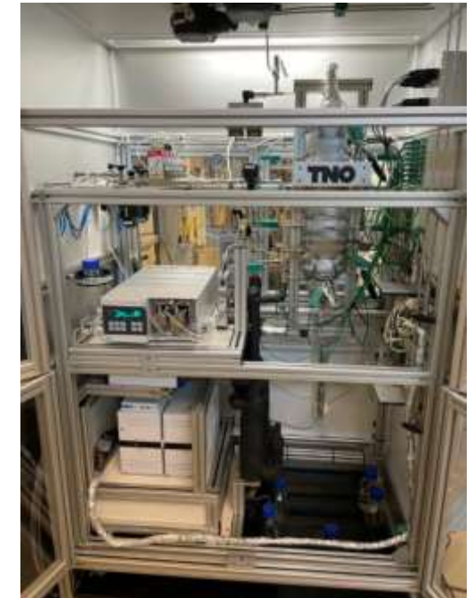
Testing SIENNA (in situ water separation reactor – for MeOH/DME)
