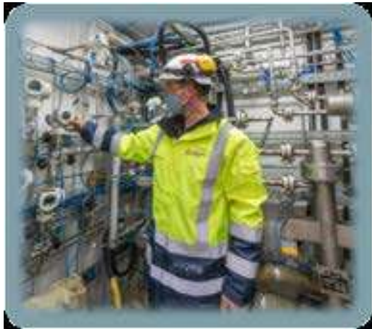
CO 2 hydrogenation catalytic tests High throughput test – 16 parallel reactors
