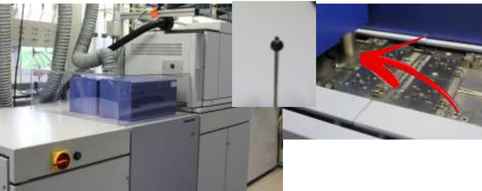
CO 2 hydrogenation catalytic tests High throughput test – 16 parallel reactors
